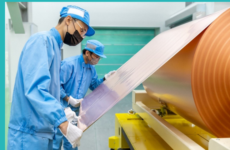
Inspecting copper foil produced at SK nexilis’ first factory in Malaysia
